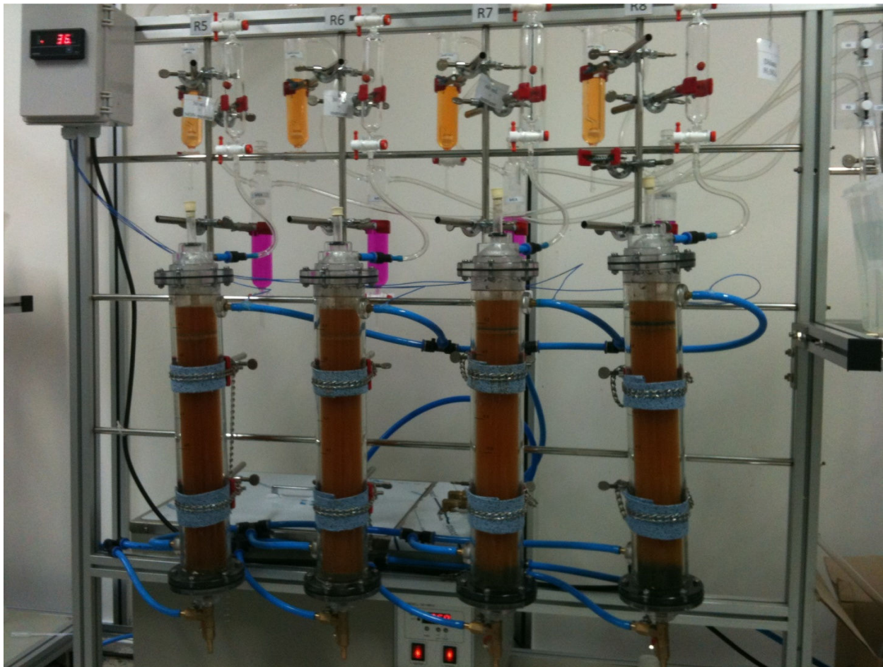
Fig. 1. Laboratory scale model fermentor for the production of Volatile fatty acids
