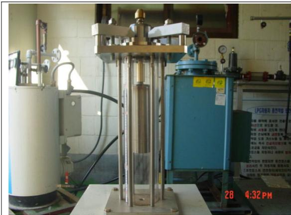
Figure 3. Performance test of a new type reliable check-floater.
