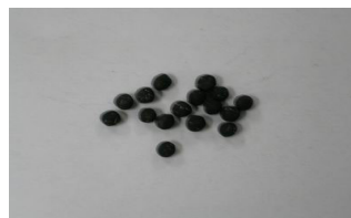
Fig.2 Prox Catalyst by Pt wet impregnation
