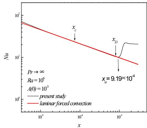
Fig.3. Deviation from laminar forced convection
