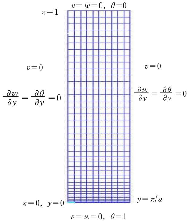
Fig. 1. Finite element meshes and boundary conditions
