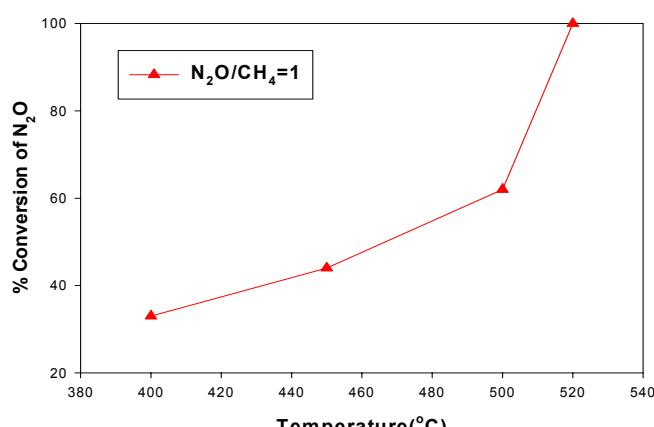
Fig. 4. Catalytic activity of FeHNZ catalyst for  $\text{N}_2\text{O}$  removal: s.v.=15,000h<sup>-1</sup>, pressure=3bar,  $[\text{N}_2\text{O}] = [\text{NH}_3] = 1,000\text{ppm}$ ,  $[\text{O}_2] = 2\%$ , in He balance.
