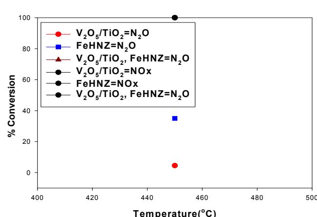
Fig. 5. Activity of the dual bed catalytic systems: s.v. = 15,000 h<sup>-1</sup>, [N<sub>2</sub>O] = [NO<sub>x</sub>] = 1,000 ppm, [NH<sub>3</sub>] = [CH<sub>4</sub>] = 1,000 ppm, [O<sub>2</sub>] = 2%, [H<sub>2</sub>O] = 1% and He balance
