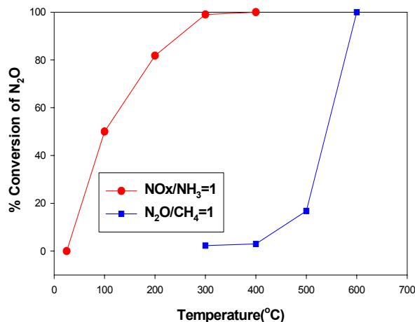
Fig. 2. Activity of FeHNZ and  $\text{V}_2\text{O}_5/\text{TiO}_2$  catalysts: s.v.=15,000h<sup>-1</sup>,  $[\text{N}_2\text{O}] = [\text{NOx}] = 1,000\text{ppm}$ , pressure=3bar,  $[\text{NH}_3] = [\text{CH}_4] = 1,000\text{ppm}$ ,  $[\text{O}_2] = 2\%$ ,  $[\text{H}_2\text{O}] = 1\%$  and He balance.
