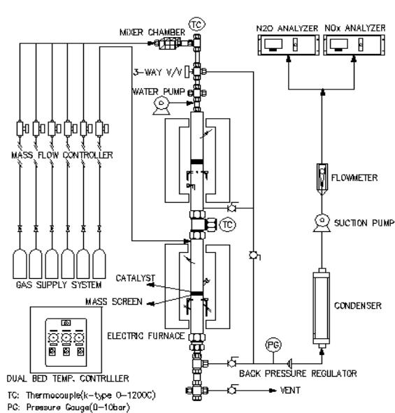
Fig. 1. Schematic flow diagram of apparatus for testing the catalysts
