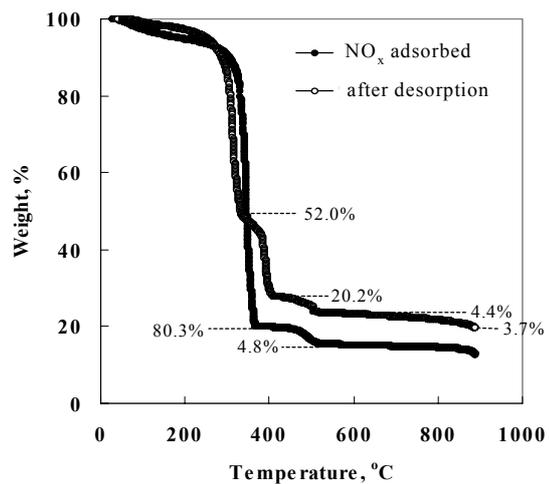
Figure 3. TGA curves after adsorption and desorption on alkaline-AC Reference
