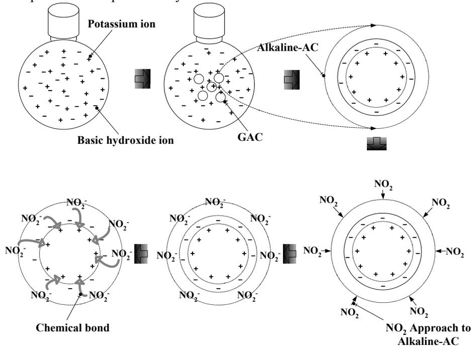
Figure 1. Predicted electrochemical status of surface from the manufacture of alkaline-AC to adsorption of NO<sub>2</sub>.
