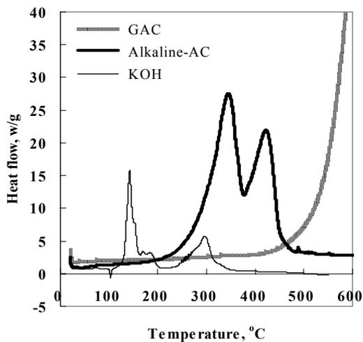
Figure 2. DSC analysis on KOH, GAC and alkaline-AC.
