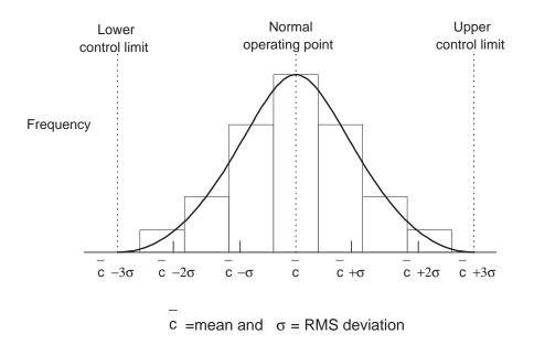
• Establish control limits based on the desired probability level  $\gamma$ . For normal distribution,
