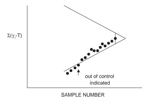
Here one can set some tolerance on the rate of rise / fall. If any leg of the V-mask crosses the plotted CUSUM values, a *mean-shift* is thought to have occurred.
