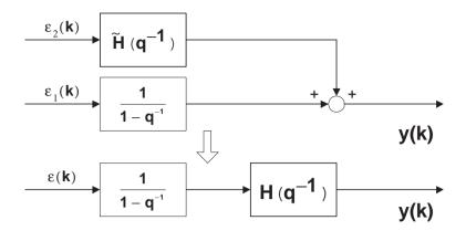
As shown above, the combined effects can be expressed as an integrated white noise colored with a filter  $H(q^{-1})$ .
