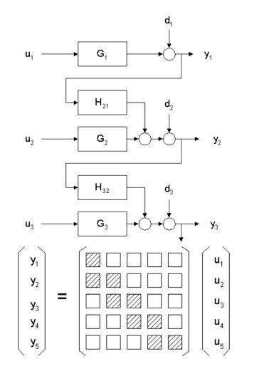
According to the input-output map,  $u_j - y_j$  pair is decoupled from others while  $u_{j-1}$  plays a measurable disturbance to  $y_j$ . Instead of treating  $u_{j-1}$  as a measured disturbance, however, it is
