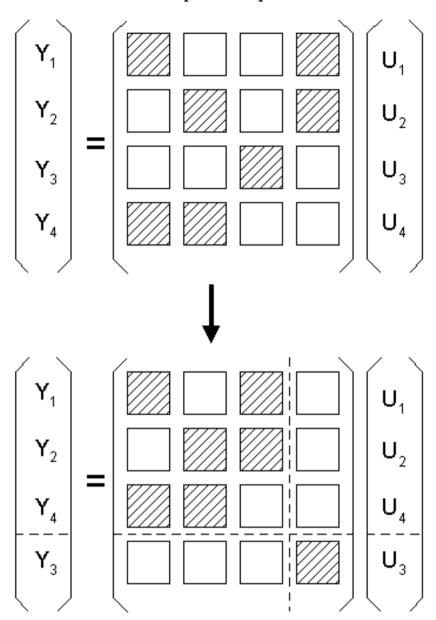
• The system can be decomposed into  $(U_1\ U_2\ U_4)-(Y_1\ Y_2\ Y_4)$  and  $U_3-Y_3$  disjoint pairs.
