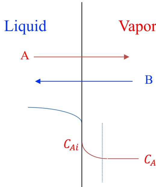
$$N_A = D_v \frac{C_{Ai} - C_A}{\delta} \left( = D_v C \frac{y_{Ai} - y_A}{\delta} \right)$$
