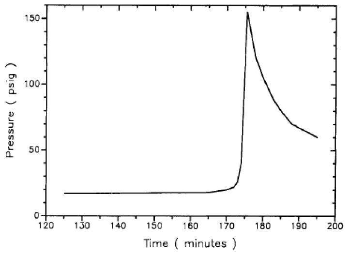
Runaway reaction pressure data acquired using the vent sizing package
