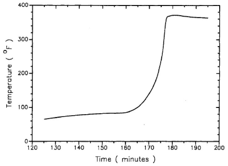
Runaway reaction temperature data acquired using the vent sizing package (VSP)
