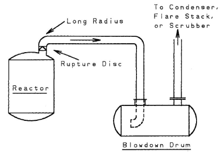
Relief containment system with blowdown drum. The blowdown drum separates the vapor from the liquid
