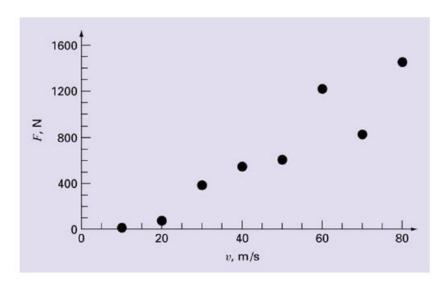
Data from wind tunnel experiments: Drag force (F) at various wind velocities
