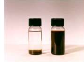
Iron oxide (left) without (right) with dextran
