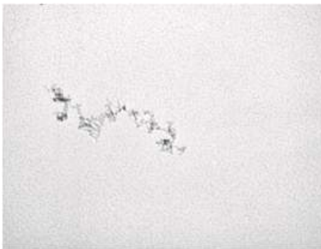
Aggregation of TiO 2 nanoparticles
