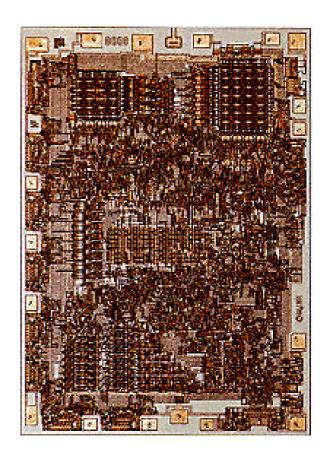
The Motorola 68000 microprocessor exhibited a processing speed far greater than its contemporaries. This high performance processor found its place in powerful work stations intended for graphics-intensive programs common in engineering.
