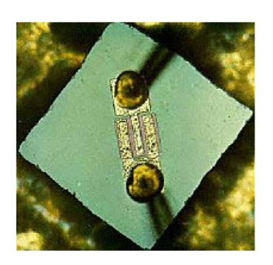
Jean Hoerni's Planar process, invented at Fairchild Camera and Instrument Corp., protects transistor junctions with a layer of oxide. This improves reliability and, by allowing printing of conducting channels directly on the silicon surface, enabled Robert Noyce's invention of the monolithic integrated circuit
