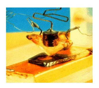
Silicon-based junction transistor, perfected by Gordon Teal of Texas Instruments Inc., brought the price of this component down to \$2.50. A Texas Instruments news release from May 10, 1954, read, "Electronic "brains" approaching the human brain. Texas Instruments Incorporated of the first commercial production of silicon transistors kernel-sized substitutes for vacuum tubes."
