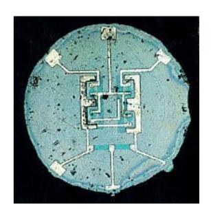
Fairchild Camera and Instrument Corp. built the first standard metal oxide semiconductor product for data processing applications, an eight-bit arithmetic unit and accumulator. In a MOS chip, engineers treat the semiconductor material to produce either of two varieties of transistors, called n-type and p-type.
