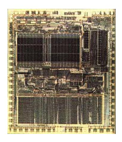
Compag beat IBM to the market when it announced the Deskpro 386, the first computer on the market to use Intel's new 80386 chip, a 32-bit microprocessor with 275,000 transistors on each chip. At 4 million operations per second and 4 kilobytes of memory, the 80386 gave PCs as much speed and power as older mainframes and minicomputers.
