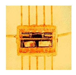
Fairchild Camera and Instrument Corp. produced the first widely accepted epitaxial gold-doped NPN transistor. The NPN transistor served as the industry workhouse for discrete logic
