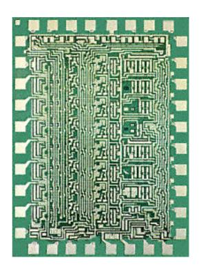
Intel's 8008 microprocessor made its debut. A vast improvement over its predecessor, the 4004, its eight-bit word afforded 256 unique arrangements of ones and zeros. For the first time, a microprocessor could handle both uppercase and lowercase letters, all 10 numerals, punctuation marks, and a host of other symbols.
