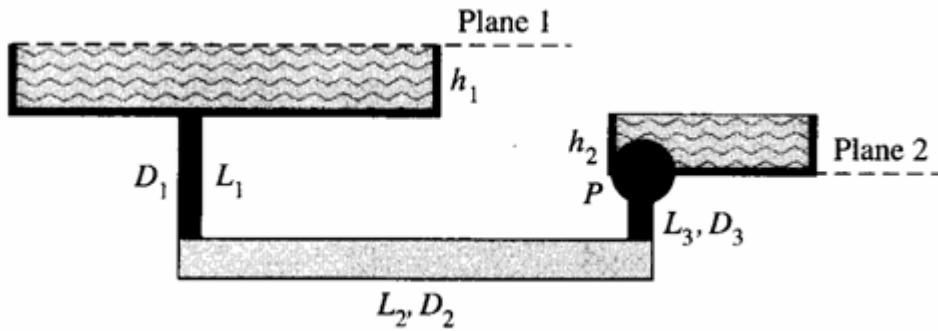
$$\begin{aligned}h_1 &= 10m, h_2 = 3m, \\L_1 &= 50m, L_2 = 300m, \\L_3 &= 1m, D_1 = 0.2m, \\D_2 &= 0.5m, D_3 = 0.03m, \\w_2 &= 60\text{kg/s}\end{aligned}$$
