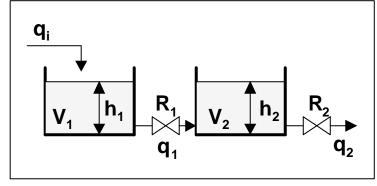
$$A_{1}\frac{dh_{1}}{dt} = q_{i} - \frac{1}{R_{1}}(h_{1} - h_{2}) \qquad A_{2}\frac{dh_{2}}{dt} = \frac{1}{R_{1}}(h_{1} - h_{2}) - \frac{1}{R_{2}}h_{2}$$
