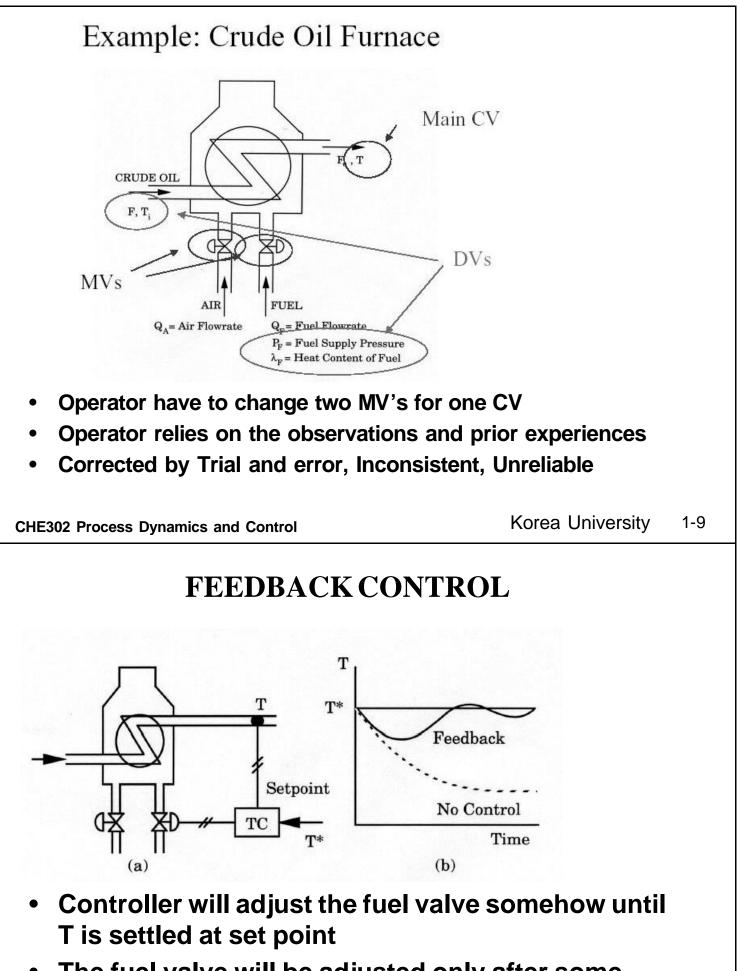
The fuel valve will be adjusted only after some change happen at the measurement
