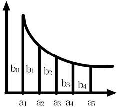
$$S = \int_{Y_{A_1}}^{Y_{A_2}} \frac{dY_A}{Y_A - Y_A^*} = \frac{1}{2}(b_0 + b_1)a_1 + \frac{1}{2}(b_1 + b_2)a_2 + \frac{1}{2}(b_2 + b_3)a_3 + \dots$$
