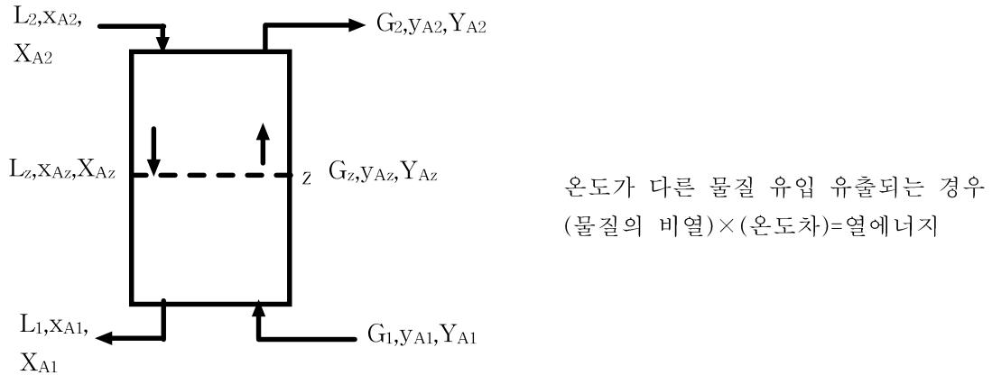
$$\text{엔탈피 수지식} : L_2 H_{L_2} + G H_G = G_2 H_{G_2} + L H_L$$
