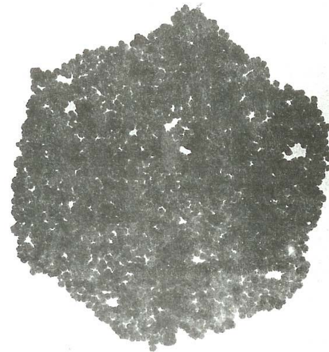
TEM of aggregate obtained by aging at 90°C for 12 h a solution of 0.015 M (NH 4 ) 2 Ce(NO 3 ) 6 , 0.064 M H 2 SO 4 , and 0.16 M Na 2 SO 4 , pH 1.1. From Hsu et al. [108].
