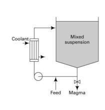
(a) Circulation of magma through an external, cooling heat exchanger
