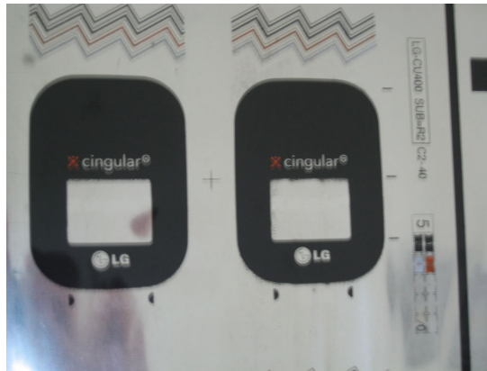
Fig. 2. The Insert PET film for the cellular-phone.
