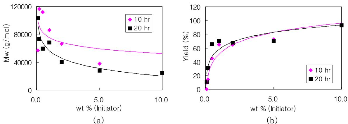
Figure 2. Variation of Molecular Weight (a) and Yield (b) of PVAc upon the Amount of Initiator for 2 Different Reaction Time at 345 bar and 338.15 K.
