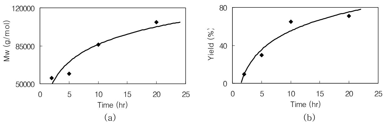
Figure 4. Variation of Molecular Weight (a) and Yield (b) of PVAc upon Reaction Time at 345 bar, 338.15 K.
