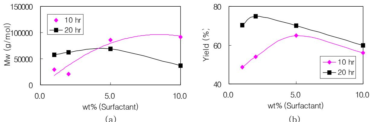
Figure 3. Variation of Molecular Weight (a) and Yield (b) of PVAc upon the Amount of Surfactant for 2 Different Reaction Time at 345 bar and 338.15 K.
