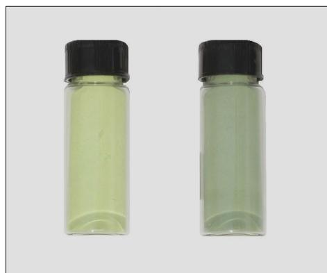
Fig. 4. The color of tungsten samples after 10 hours at  $650^\circ\text{C}$  under the helium condition.
