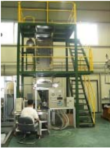
Fig. 1. Photo of cartridge filter test unit.
