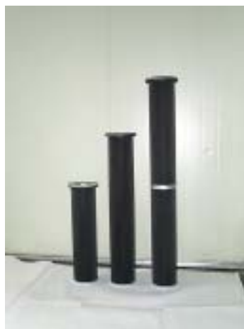
Fig. 3. Cylindrical pleated filters used in the present study. (Left - 600 mm; middle-900 mm; right-1200 mm in length)
