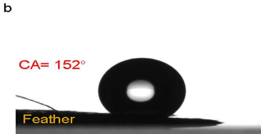
Figure 5 | Enhanced hydrophobicity in feather and feather-inspired photonic crystal structure. (a), Neck feathers exhibit superhydrophobicity due to presence of structural hierarchy. (b), Contact angle measurement of a single mallard feather. (c), Our photonic crystal surface enhances the intrinsic hydrophobicity of PVDF film (see Figure S5) by increasing surface roughnesses. (d), The nanoscale surface pattern observed on step III structures and the alignment of the fiber arrays both contribute to surface superhydrophobicity. (e), The water contact angle is measured to exceed 165° for this particular array.
