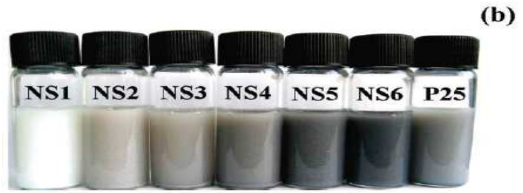
Figure 4. UV-vis absorbance spectra (a) and the corresponding photos (b) of suspensions in water for the samples prepared at R_{Pt} = 0 (NS1), 0.5 (NS2), 1 (NS3), 2 (NS4), 4 (NS5), and 6 (NS6) and P25 prepared at R_{Pt} = 2 without F.
