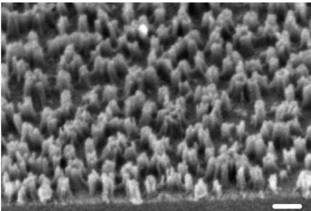
(30 to 65 nm in spacing / 30 to 100 nm in height)
