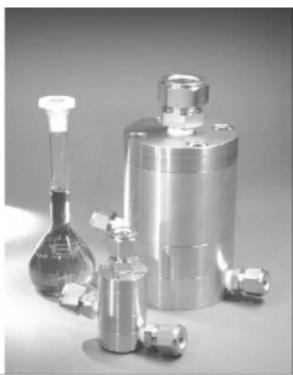
[ 1] Glass devices as examples for micromixers (left; typical flow rate: up to 3 dm $^3$  h $^{-1}$ ) and microstructured high throughput mixers (right; typical flow rates: up to 1 and 5m $^3$  h $^{-1}$ , respectively, at a pressure drop of 3 bar).
