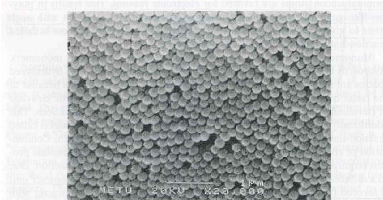
**Figure 4-53.** Monodisperse silica spheres with a diameter of about 0.2  $\mu\text{m}$  made by the Stöber process.
