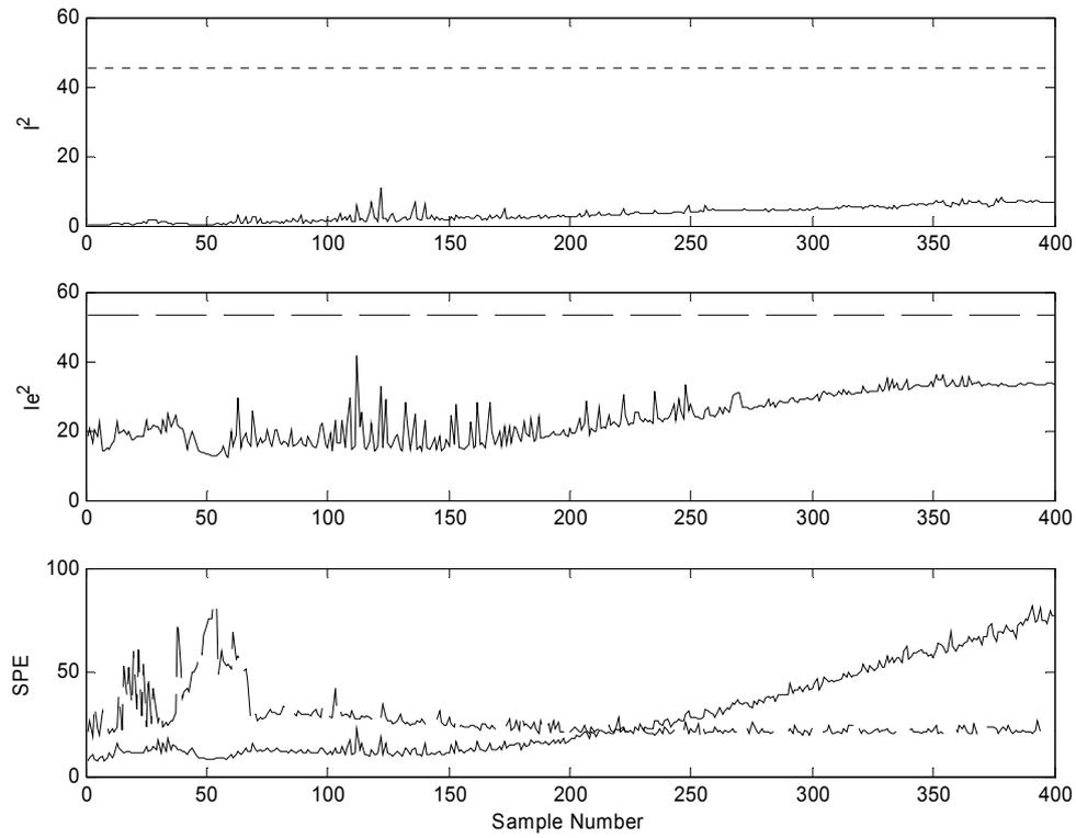
그림 12. On-line MICA monitoring charts for an *abnormal* test batch in which the substrate feed rate was decreased by 10% at sample 50:  $I^2$ ,  $I_e^2$  and  $SPE$  charts with 99% control limits.
