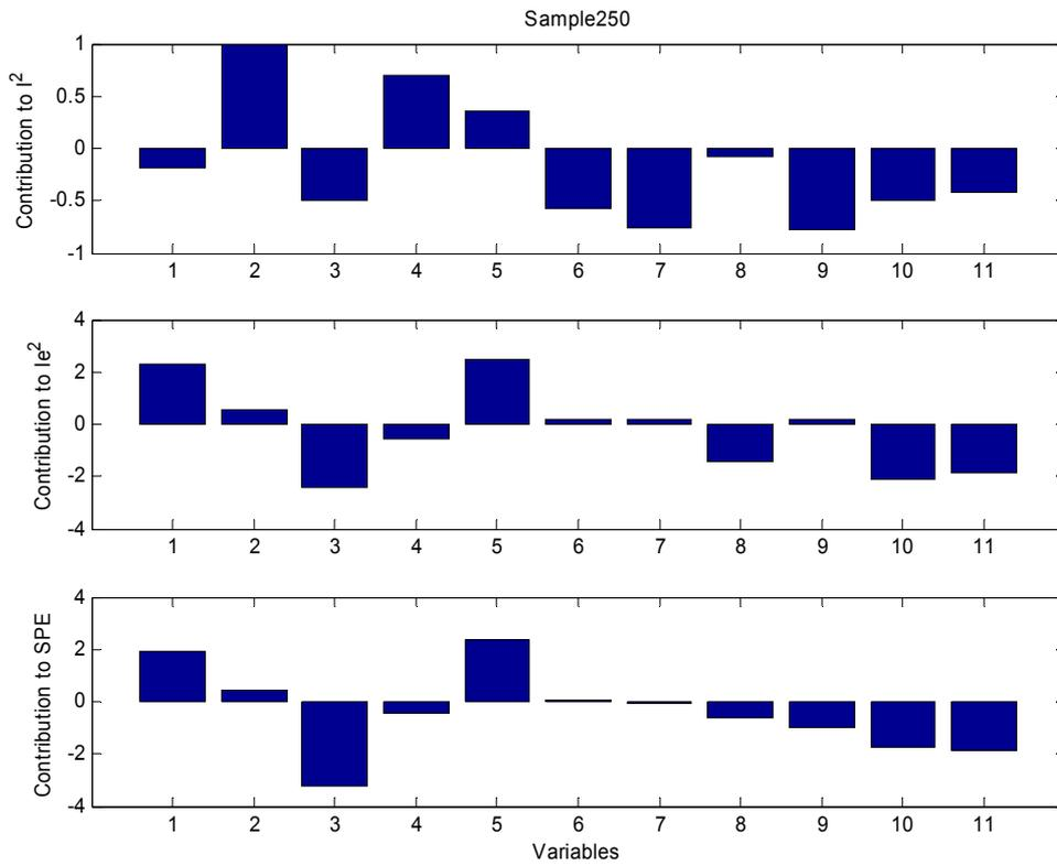
그림 13. Contribution plots at sample 200 of the MICA model for the *abnormal* test batch in which the substrate feed rate was decreased by 10% at sample 50:  $I^2$ ,  $I_e^2$  and  $SPE$  contributions.
