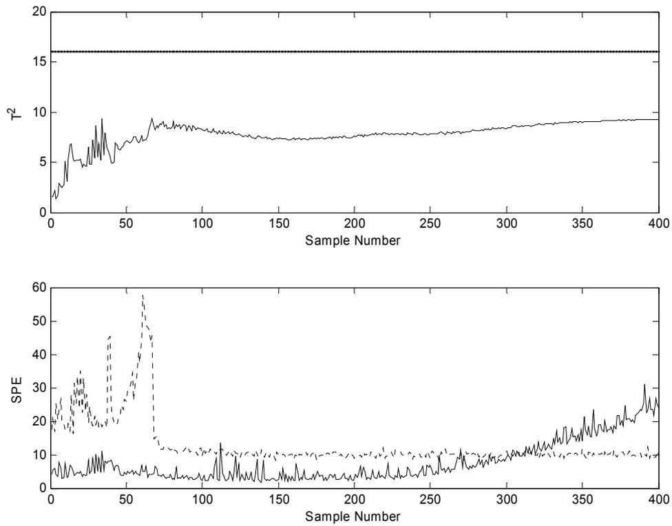
Figure 8. On-line MPCA monitoring charts for an *abnormal* test batch in which the substrate feed rate was decreased by 10% at sample 50:  $T^2$  and  $SPE$  charts with 99% control limits.
