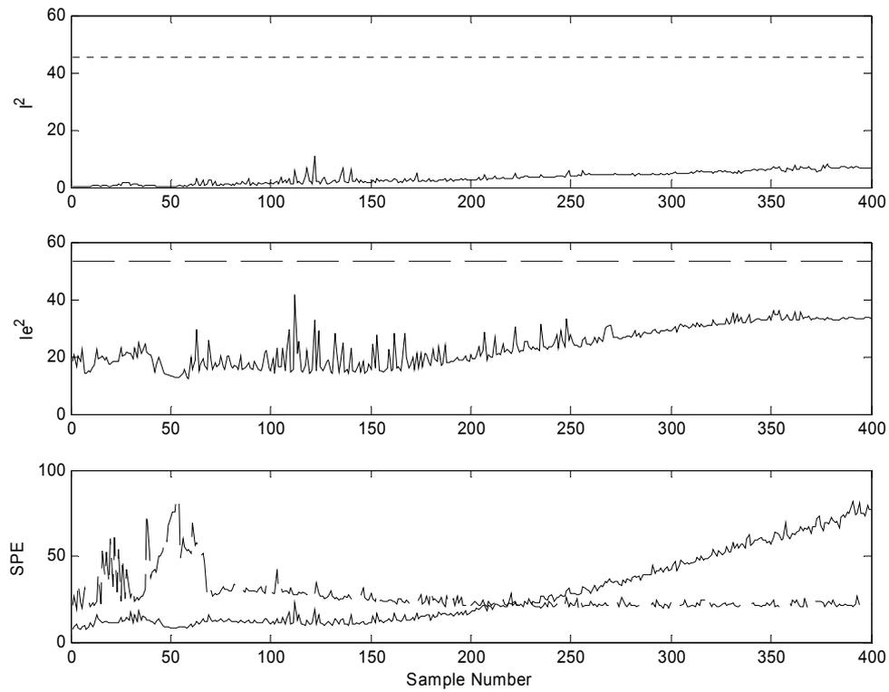
Figure 9. On-line MICA monitoring charts for an *abnormal* test batch in which the substrate feed rate was decreased by 10% at sample 50:  $I^2$ ,  $I_e^2$  and  $SPE$  charts with 99% control limits.
