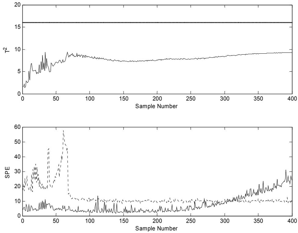
그림 11. On-line MPCA monitoring charts for an *abnormal* test batch in which the substrate feed rate was decreased by 10% at sample 50:  $T^2$  and  $SPE$  charts with 99% control limits.
