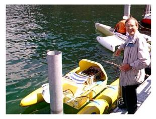
A "300 W Powerpack" prototype has been designed at PSI, in Villigen, and has been duplicated at the Grenchen School of Engineering. The **Hydroxy300** from MW-Line is a two passengers electric boat with a cruising speed of **12 km/h**, while the one seat Hydroxy100 cruises at only 4 km/h. The "Fuel cell fleet" has been demonstrated on June 21<sup>st</sup>. More ergonomically control systems are under development. In view of Low Cost prospect, fluorine free membranes are currently evaluated.
