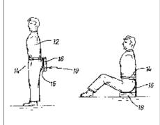
UK Patent Application No. GB2267208. A portable seat which you wear on a waist-belt. The seat cushion 18 is pivotable between a stowed position (left drawing) and a seating position in which it hangs down so that you can sit on it (right drawing).
