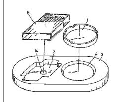
UK Patent Application No. GB2251542. An ashtray which warns you to quit smoking. When you pick up the box of matches 5 from the holder 2, light passes through a hole 14 to a photocell. This activates an audible warning device.
