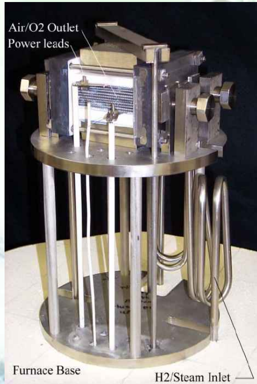
Ten-cell electrolysis mounted for testing at INEEL
