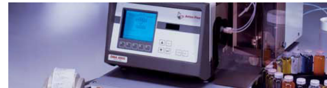
Anton Paar Density Meter : Oscillating U-tube method
