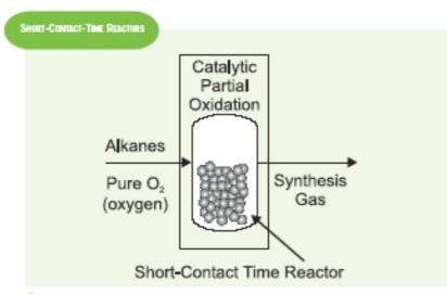
Oxygen is combined with simple alkanes (methane, ethane) over a catalyst at high temperatures to produce synthesis gas.
