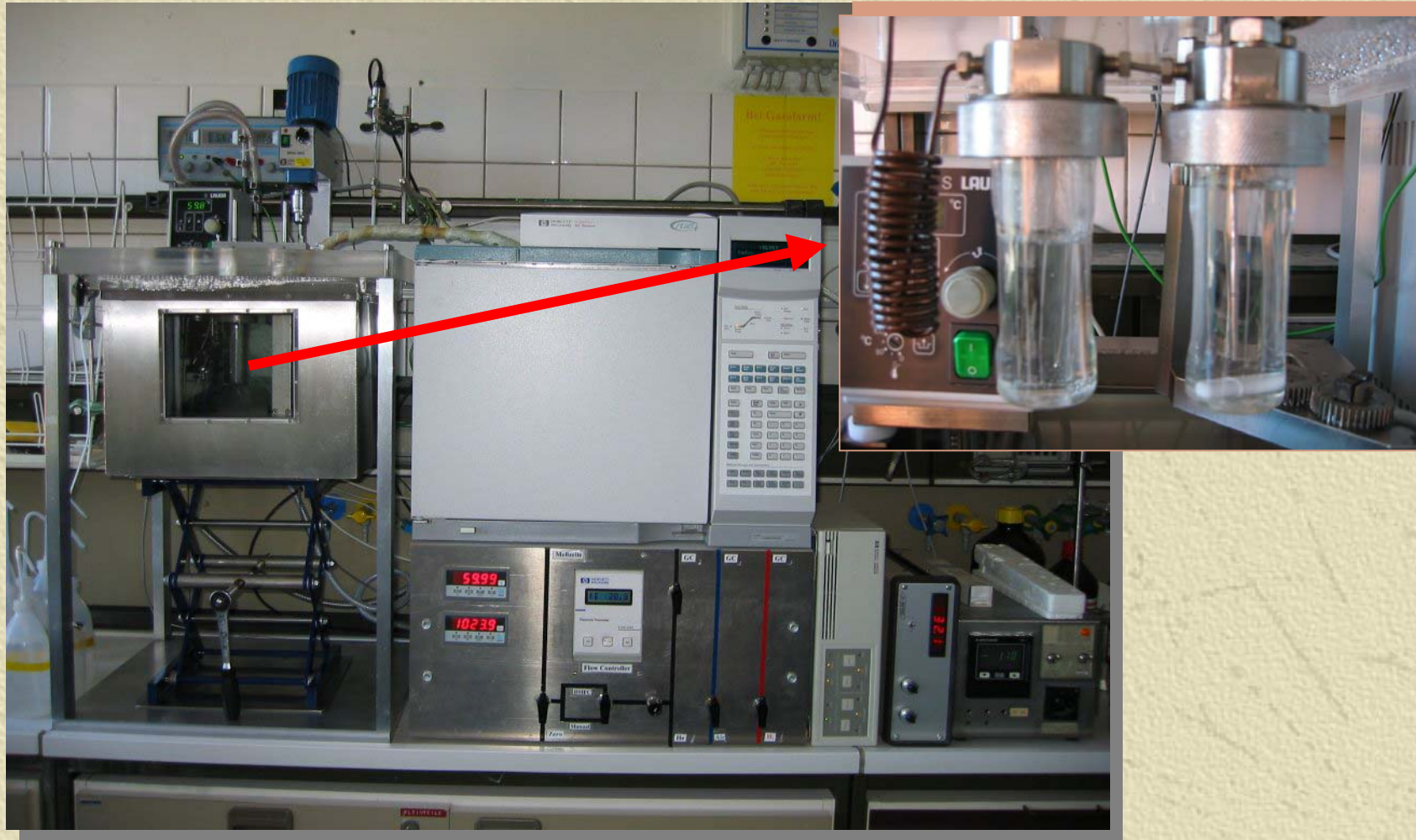
Figure. Picture of the dilutor system for measuring \gamma^\infty .
