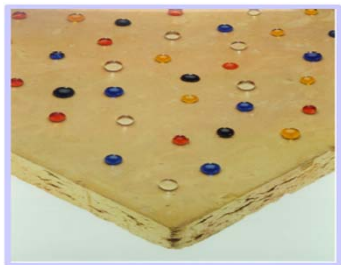
Porous surface protection
