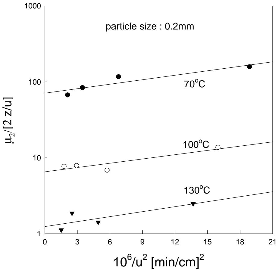
**Fig. 6 Second Moment Plot of Methanol on Activated Carbon**
