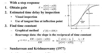
$\theta = 1.3t_{35.3\%} - 0.29t_{85.3\%} \quad \tau = 0.67(t_{85.3\%} - t_{35.3\%})$
